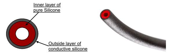
Both types can in an economical way be delivered spliced into endless O-rings by use of the patented Compashield Splicing Tool. This can in many application be an advantage to make assembly easier and to ensure that no gap can occur over time.
